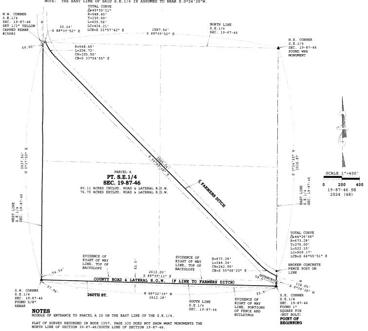
USED TOP OF BACKSLOPE AS EVIDENCE OF LATERAL RIGHT OF WAY.
