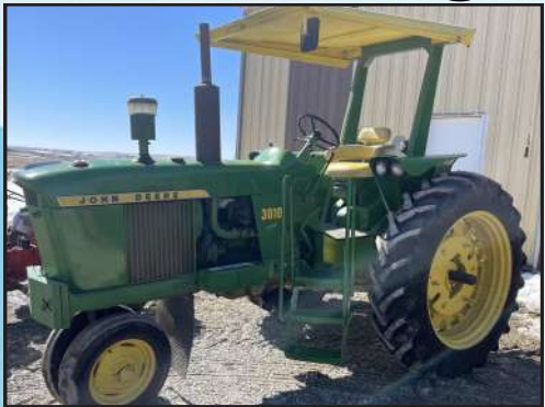
1963 JOHN DEERE 3010. 5,936 HRS. SYNCHRO TRANSMISSION. GAS. NARROW FRONT END. CANOPY. 4 TOTAL REAR WEIGHTS. FRONT 3 STEP ACCESSORY. 3PT. 2 HYD. STARTS AND RUNS WELL. SN:39641
